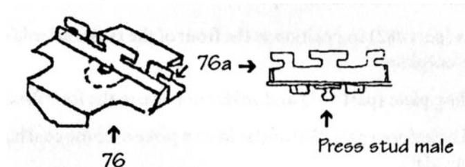
4.2 Fold up the movement limiter pieces on a bogie pivot plate (part #76), fold the ends of a bogie retaining plates (part #76a) to 90° and insert into the pivot plate as shown above. Retain by twisting the tabs and secure by soldering making sure the retaining plate is at 90° to the pivot plate.
