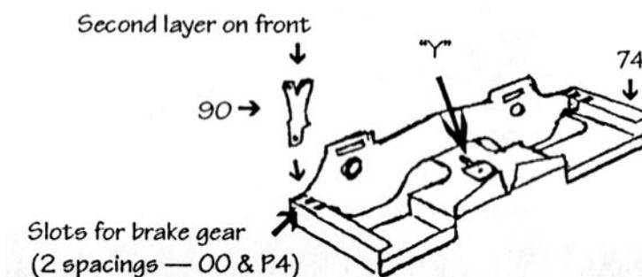
4.4 Press out the rivet detail on the bogie sideframes (part #74).
