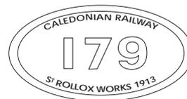
Works plates were not originally carried by these engines as the information was incorporated in the number plate however the L.M.S. affixed small oval works plates with raised lettering which were fitted to the splasher. These were rather anachronistically lettered as illustrated below with the third row being the year of building — i.e. many a year before the formation of the L.M.S. !
