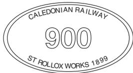
Works plates were not originally carried by these engines as the information was incorporated in the number plate however the L.M.S. affixed small oval works plates with raised lettering which were fitted to the splashers. These were rather anachronistically lettered as illustrated below with the third row being the year of building — i.e. many a year before the formation of the L.M.S. !
